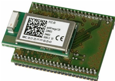
Figure 61: deRFmega128-22T00 adapter board with radio module deRFmega128-22M00 / deRFmega256-23T00 adapter board with radio module deRFmega256-23M00
