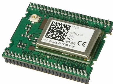
Figure 62: deRFmega128-22T02 adapter board with radio module deRFmega128-22M10 / deRFmega256-23T02 adapter board with radio module deRFmega256-23M10
