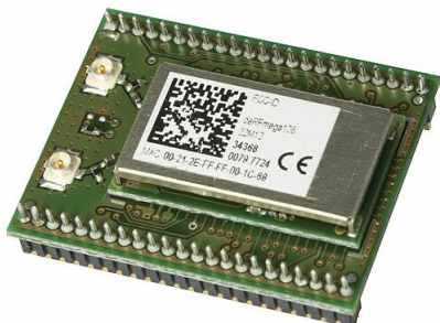
Figure 63: deRFmega128-22T13 adapter board with radio module deRFmega128-22M12 / deRFmega256-23T13 adapter board with radio module deRFmega256-23M12
