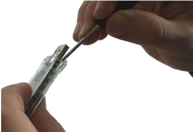
Figure 65: Removal of the plastic enclosure
