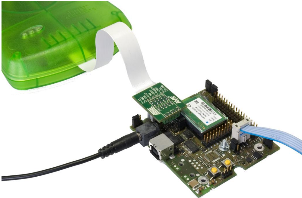
Figure 53: AVR JTAGICE mkII connected to deRFmega128 plugged onto a deRFnode
