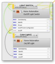
comprehensive monitoring, control and commissioning capabilities based on the ZigBee PRO specification. The application core is kept completely generic and is therefore not limited to a specific application profile. All ZigBee application specifics like devices, profiles and clusters are described in a XML file. Based on this information, the deCONZ application can generate a full functional graphical user interface for each device and any application.
