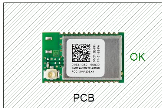
Figure 9-6: Placing in the centre with RF pad antenna
