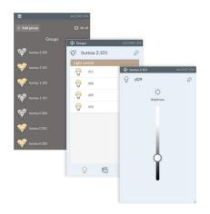
The Phoscon App allows professional management of light installations with up to 200 devices. The ZigBee mesh-network can be used over a wide area with several floors for lights, switches and sensors. The Phoscon solution is therefore not only suitable for usage in the home, but also to control office buildings or industrial halls.
